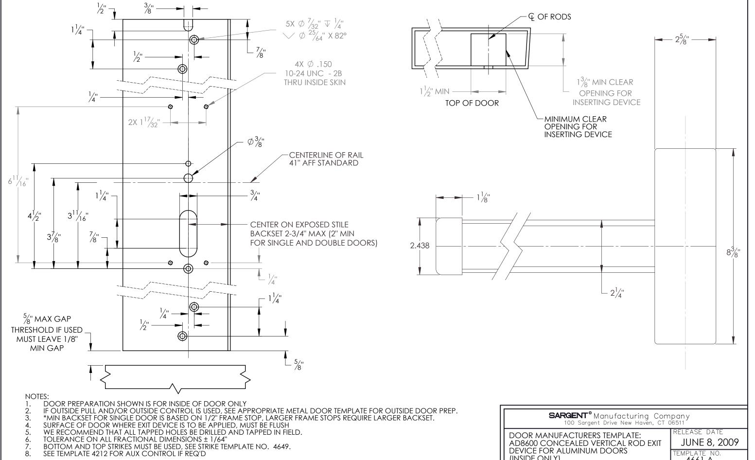
DOOR MANUFACTURERS TEMPLATE: AD8600 CONCEALED VERTICAL ROD EXIT DEVICE FOR ALUMINUM DOORS (INSIDE ONLY)
