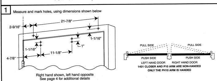
Pre-drill - 3/32" holes for self tapping screws or #16 drill for #12-24 tap for machine screws
