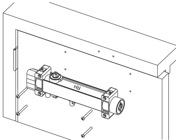
**B** ATTACH FOOT TO FRAME WITH PIVOT AWAY FROM HINGE.
