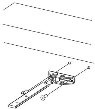
**C** INSTALL MAIN ARM TO SPINDLE AND SECURE WITH SCREW AND WASHER AS SHOWN. OPEN DOOR INSERT RETANGULAR ROD INTO SWIVEL ARM THEN CLOSE THE DOOR AND TIGHTEN ARM SCREW SECURELY WHEN SWIVEL ARM IS AT RIGHT ANGLE TO DOOR.
