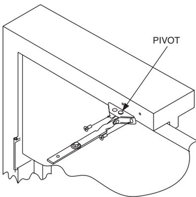
**C** ATTACH ARM WITH INDEX MARK ON SPINDLE ALIGNED AS SHOWN. SECURE WITH SCREW AND WASHER. INSERT ROD END INTO SWIVEL ARM AND TIGHTEN ARM SCREW AS SHOWN BELOW.
