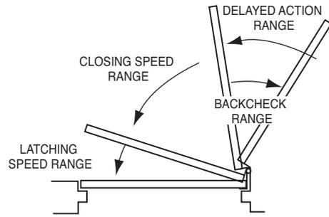
**A** REGULATING DOOR SPEED AND LATCHING SPEED AS NEEDED.
