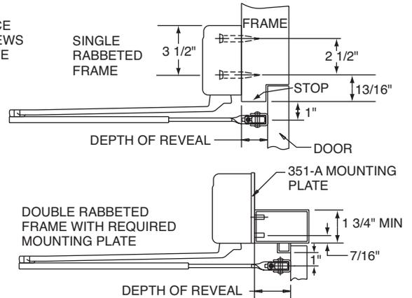
**A** INSTALL DOOR CLOSER TO FRAME WITH SPRING ADJUSTMENT NUT AWAY FROM HINGE.
