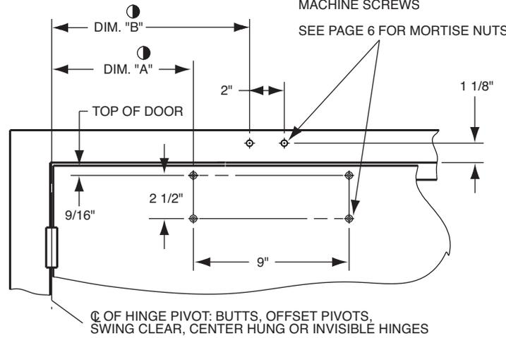
**A** INSTALL DOOR CLOSER TO DOOR WITH SPRING ADJUSTMENT NUT AWAY FROM HINGE.
