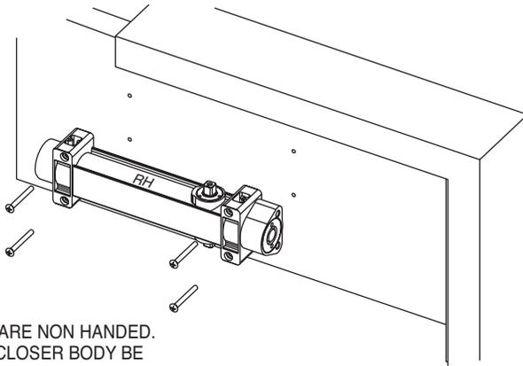
NOTE: 351 CLOSER BODIES ARE NON HANDED. IT IS IMPORTANT THAT THE CLOSER BODY BE MARKED WITH "RH" SYMBOL AT TOP, FOR RIGHT HAND DOORS. "LH" SYMBOL AT TOP FOR LEFT HAND DOORS.
