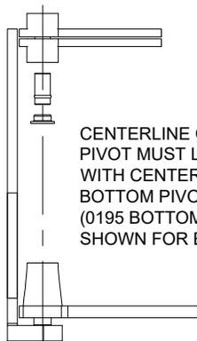
CENTERLINE OF TOP PIVOT MUST LINE UP WITH CENTERLINE OF BOTTOM PIVOT/CLOSER (0195 BOTTOM PIVOT SHOWN FOR EXAMPLE).
