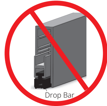
Figure 3 - Improper Drop Bar This shows an improper drop bar protruding from the end of the case. The drop bar should be flush at both ends.
