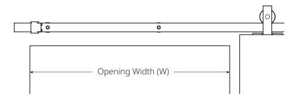
Figure 6: Measure the Width of the Opening (W)
