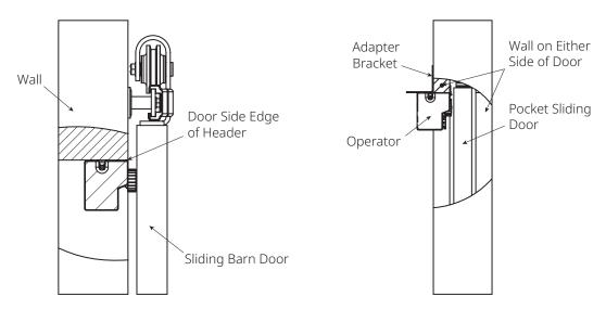
Figure 12: Sidewall Mount Sliding Door
