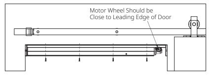
Figure 15: Mount the Unit Using the Provided Fasteners or Other Appropriate Fasteners
