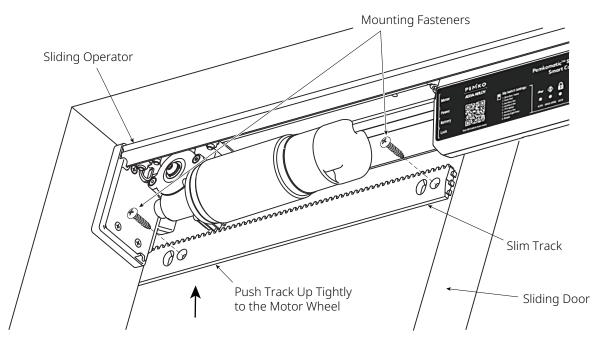
Figure 18: Mount the Track While Pushing it Up Tightly to the Motor Wheel
