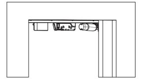
Fig 2: Overhead Mount/Pocket Door Sliding System
