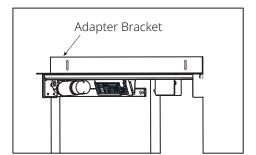
Figure 3: Overhead Mount/Pocket Door System with Adapter Bracket
