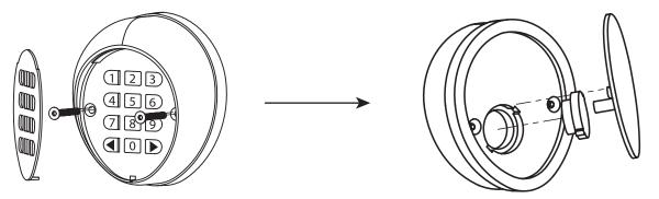
Figure 22: Install 2 CR2032 Batteries in the Keypad
