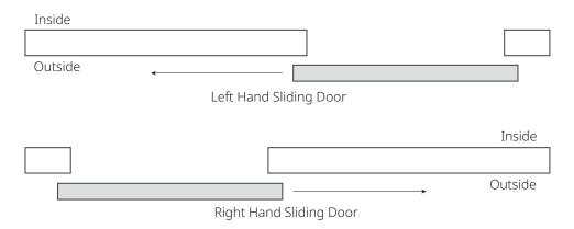
Figure 8: Sliding Door Handing Guide
