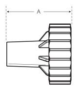
Figure 5: Measure Motor Wheel Length 'A'
