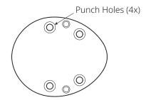
Figure 23: Punch 4 Holes for Mounting Keypad Using Fasteners
