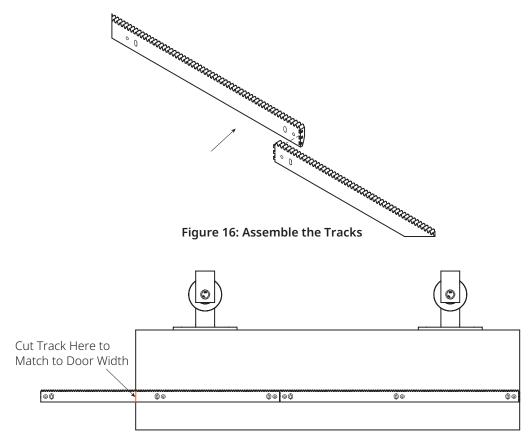
Figure 17: Length of Track = Width of the Door
