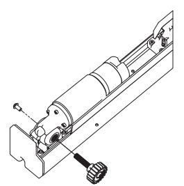
Figure 10: Remove the Motor Wheel
