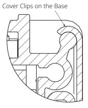
Figure 29: Clip the Cover to the Top of the Base
