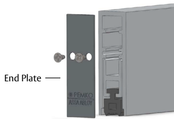
Figure 4 - Properly Installed End Plate
