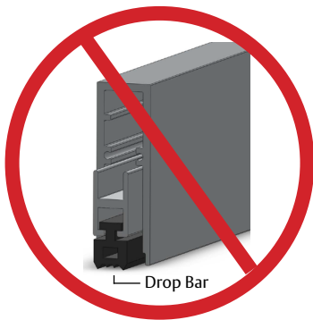
Figure 3 - Improper Drop Bar
