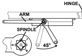
4. Close door & rotate closer spindle 45° toward hinge / pivot.
